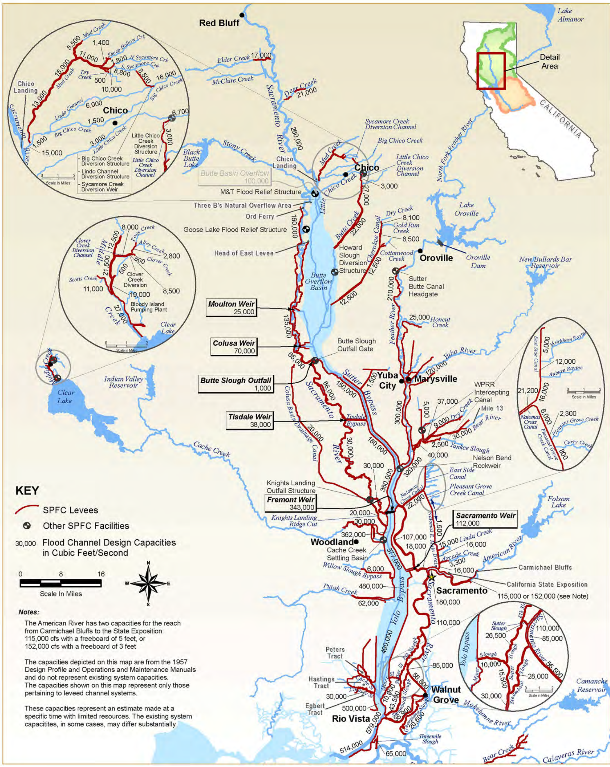
Figure 3-2. Design Flood Flow Capacities Within the Sacramento River, Bypasses, and Major Tributaries and Distributaries in the Sacramento River Basin
