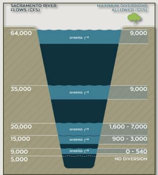
\*Depending on water year type and fish presence \*\*9,000 cfs is the maximum diversion allowed, starting when the river is at 35,000 cfs.
